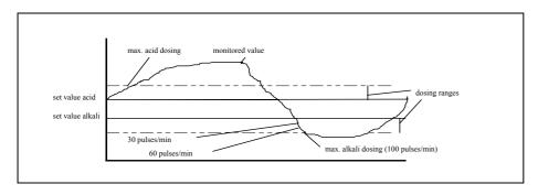
The dosing range is used to control the operation of the dosing relay whenever a difference occurs between the set value and the monitored value. Dosing range is selected in set-up mode.
