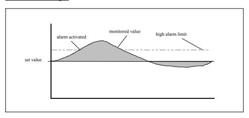
A high alarm occurs whenever the monitored value of the appropriate channel exceeds the user determined limit.
