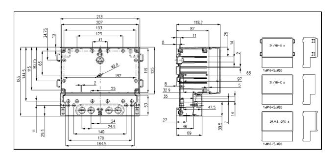
The enclosure has special made cut-outs for Autodos 5000 and the drawing below show these.
