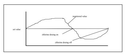
As long as the monitored value exceeds the set value then chlorine dosing is inactive. If the chlorine level falls below the set value then chlorine dosing commences and will continue until the chlorine level equals or exceeds the monitored value.
