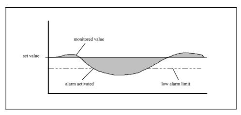
A low alarm occurs if the monitored value of the appropriate channel is below the user determined limit.
