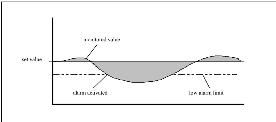
A low alarm occurs if the monitored value of the appropriate channel is below the user determined limit.
