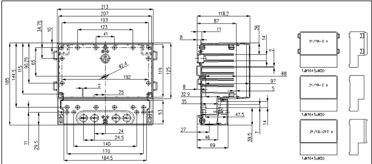
The enclosure has special made cut-outs for Autodos 2000 and the drawing below show these.
