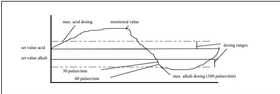
The dosing range is used to control the operation of the dosing relay whenever a difference occurs between the set value and the monitored value. Dosing range is selected in set-up mode.
