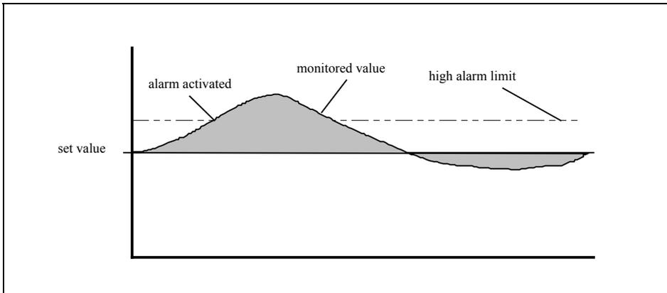
A high alarm occurs whenever the monitored value of the appropriate channel exceeds the user determined limit.
