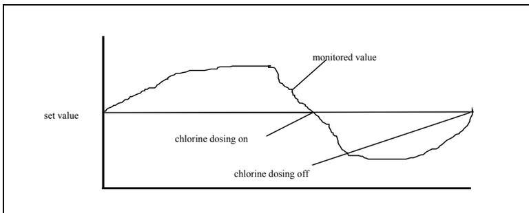
As long as the monitored value exceeds the set value then chlorine dosing is inactive. If the chlorine level falls below the set value then chlorine dosing commences and will continue until the chlorine level equals or exceeds the monitored value.
